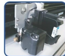
Knife Cutting & HP45 Print Head
